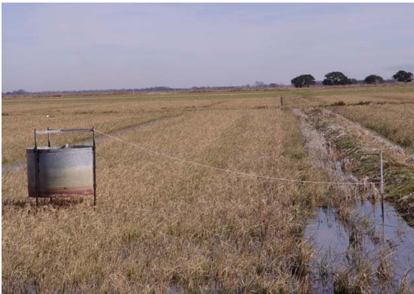
Figure 1. A drop sampler, set and ready to trip with a slight tug on the rope from the levee. Crawfish are retrieved by pumping out the water from the caisson while the cylinder walls are in contact with the mud bottom, exposing crawfish trapped within.
