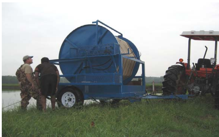
Figure 8. Tractor (43hp) used to pull the trawl using a power take-off driven hydraulic pump.
